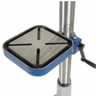
Cast Iron Tilting-Rotating Table
