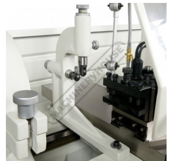
Travelling Steady With Roller Guides
