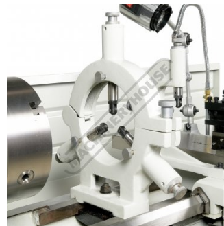
Fixed Steady With Roller Guides
