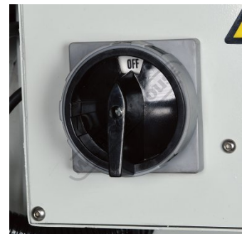
Main Isolation Switch
