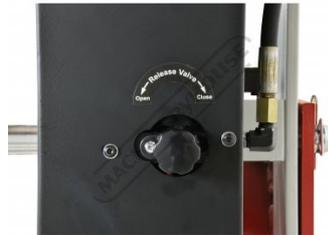
Release valve for hydraulic pump
