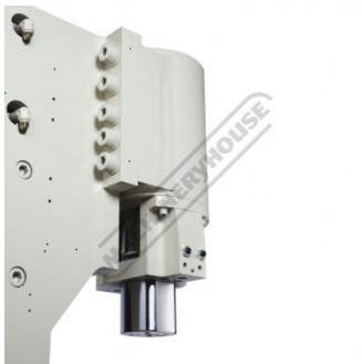
Keyed Punch Ram For Shaped Tool Alignment
