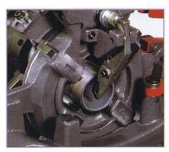
Die-Head has automatic profiling system to reduce cutting resistance.
